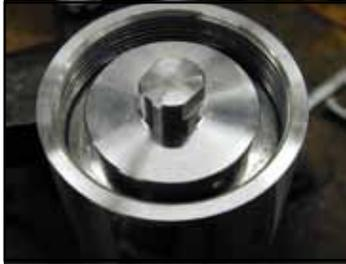
14. Install the spring and upper spring guide onto the lower spring guide.
