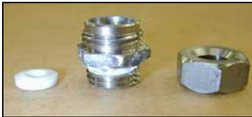
1. Inspect the Teflon soft seat insert. There can be no burrs, cuts, or scratches in the ID sealing area of the insert.
