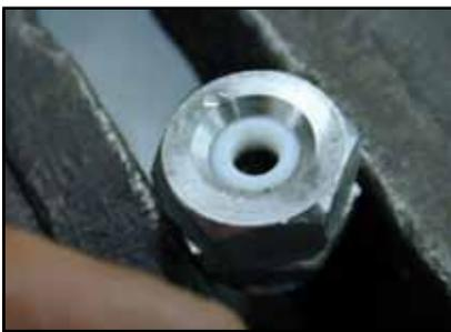
4. Apply liquid Teflon (Loctite 567) to the exposed threads of the seat assembly.
