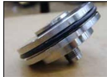
10. Install the plug, plug spring, follower, and stem seal into the piston in order as shown below.
