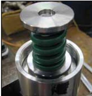
15. Use anti-seize and generously coat the spring housing threads.
