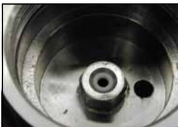
6. Lube the piston and cylinder o-rings with Dow Corning grease.
